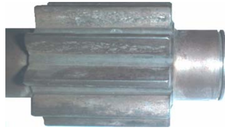
Fig. 4 Pitting of gear teeth flanks
