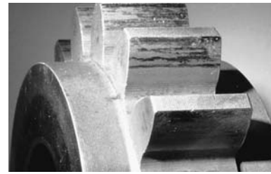
Fig. 3 Micropitting of gear teeth
