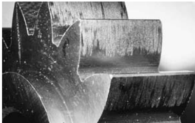
Fig. 2 Scuffing of gear teeth
